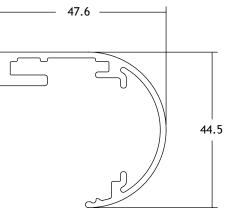
Bullnose Reflector Shell Available for 9.5mm and 6.4mm glass
