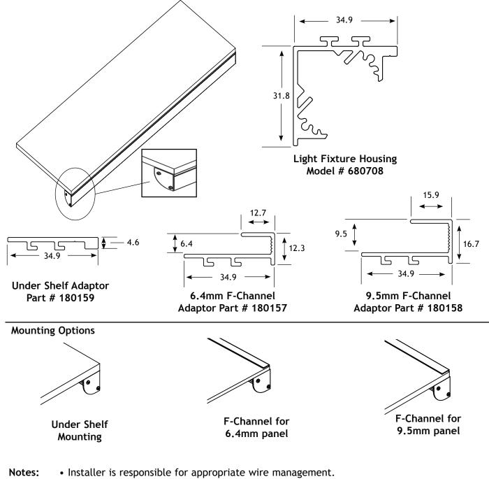
• Stylmark LED Shelf Edge is a ETL Recognized Component.
