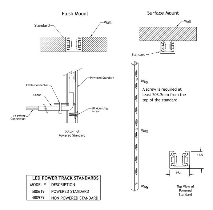
**Notes:** • LED Power Track Shelf utilizes one powered and one non-powered Stylmark standard, ranging in height from 457.2mm to 2438.4mm.
