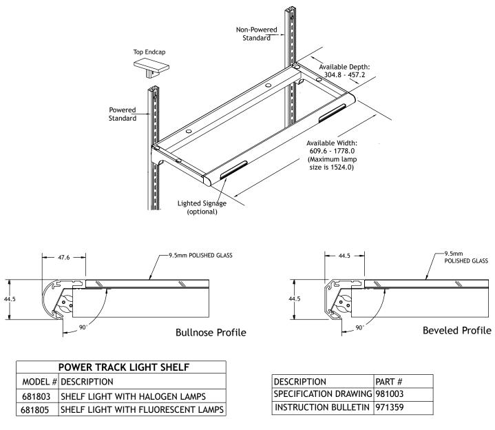
Notes: • Depth does not include reflector dimensions (see page 18 for reflector dimensions).
