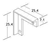
Steel Miter Bracket for Reflector Shells
