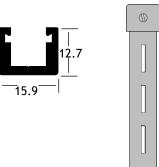
Part # 450013\* Wall Standard Used for designs requiring wall mounted standards. Comes with predrilled and countersunk holes every six inches.
